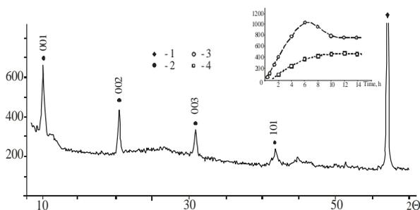
**Fig. 1.** XRD data of hydroxysulfate Green Rust II (GR(SO<sub>4</sub><sup>2-</sup>)) sample: 1 – α-Fe<sup>0</sup>, 2 – GR(SO<sub>4</sub><sup>2-</sup>); the kinetic of reflection intensity the planes of GR(SO<sub>4</sub><sup>2-</sup>): 3 – (001), 4 – (002) on the additional graph
