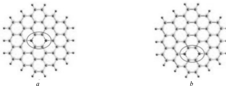
Fig. 3. PAM C_{52}N_2H_{18} with different localization (allocated by ovals) of the atoms of the nitrogen (or boron): a – in the central part of the molecule, b – at its periphery
