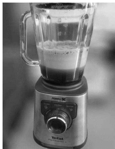
Fig. 1. Scheme of the production of graphene in a kitchen blender using PVP aqueous solution
