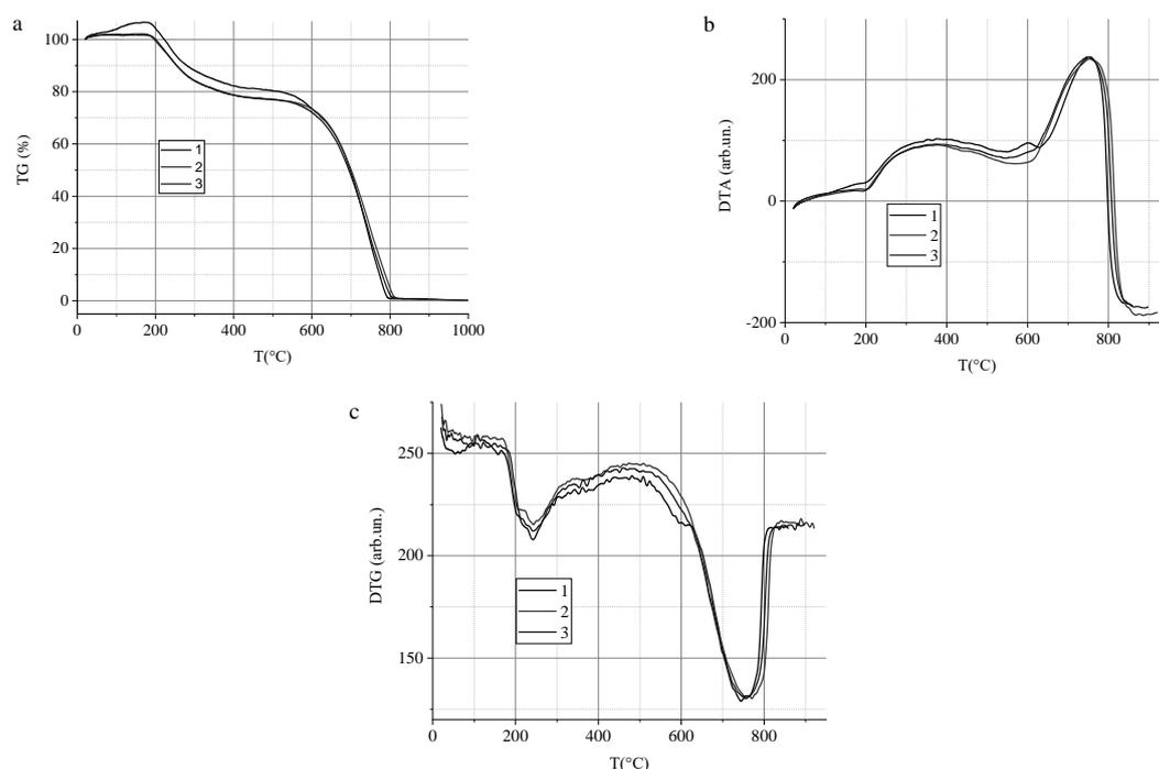
**Fig. 2.** Thermogravimetric analysis: *a* – TG; *b* – DTA; *c* – DTG, samples of natural graphite oxidized and purified: 1 – oxidation, additional purification with bifluoride; 2 – oxidation, post-cleaning with bifluoride, Trilon B; 3 – oxidation, additional cleaning with Trilon B, bifluoride
