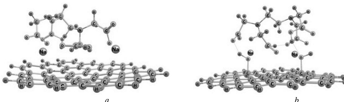
Fig. 4. Interaction of Trilon B with native and oxidized graphene surface
