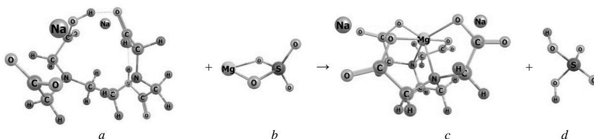
**Fig. 5.** Equilibrium geometry of the components of the reaction of Trilon B (*a*) with magnesium sulfate (*b*) to form a chelate complex of Trilon B with magnesium cation (*c*) and sulfuric acid (*d*)
