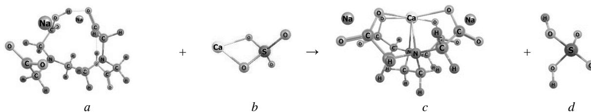
**Fig. 6.** Equilibrium geometry of the reaction components of the interaction of Trilon B (*a*) with calcium sulfate (*b*) with the formation of a chelate complex of Trilon B with a calcium cation (*c*) and sulfuric acid (*d*)
