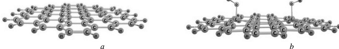
Fig. 3. Models of the native (a) and oxidized form (b) of the graphene-like plane
