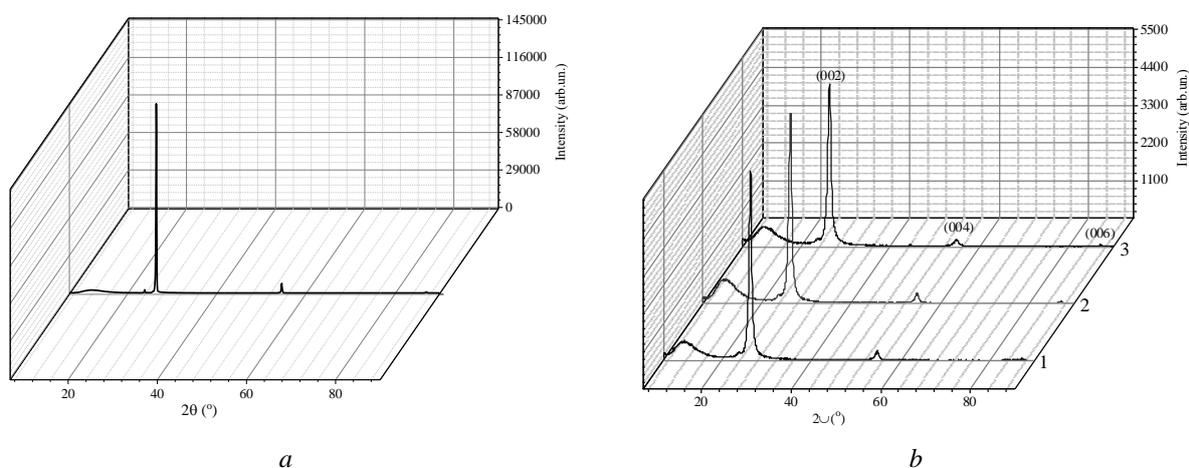
**Fig. 1.** X-ray diffraction spectra: *a* – original natural graphite; *b* – oxidized and purified samples: 1 – with ammonium bifluoride; 2 – ammonium bifluoride, Trilon B; 3 – Trilon B, ammonium bifluoride
