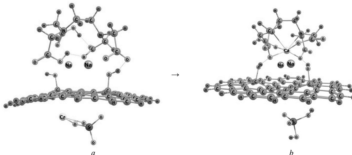
**Fig. 8.** Equilibrium geometry of complexes of starting substances (*a*) and reaction product (*b*) interaction of calcium sulfate with Trilon B on the surface of an oxidized graphene-like plane
