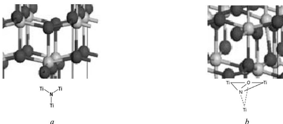
**Fig. 2.** Models for incorporated nitrogen: *a* – substitutional nitrogen (N<sub>s</sub>) and *b* – interstitial nitrogen (N<sub>i</sub>)
