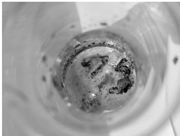
Fig. 7. Removal of crude oil from water surface with CC-Fe sample
