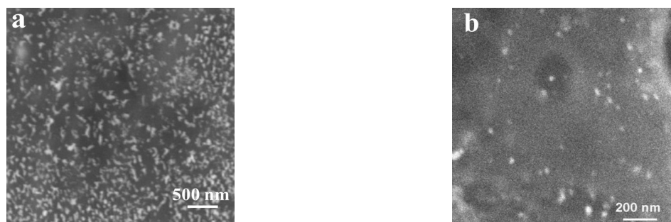
Fig. 5. SEM image of a – Ag/cotton and b – Ag/Cu cotton fabrics
