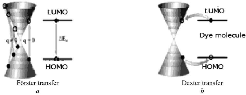
Fig. 2. Schematic illustrate of the (a) Förster and (b) Dexter energy transfer in functionalized graphene. The Dirac cone represent the electronic band structure of graphene, while the electronic states of the dye molecules are described by a two level (HOMO-LUMO) momentum independent system [16]
