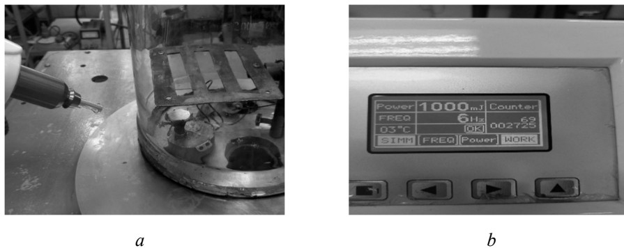
Fig. 4. Schematic representation of ( a ) pulsed laser deposition setup, ( b ) the laser energy power (1000 mJ) with frequency at 6 Hz
